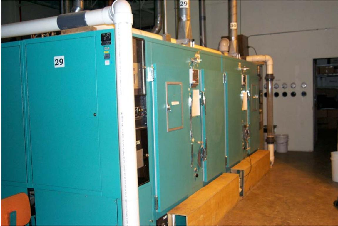
Figure 2. Six-chamber exposure system at ARC, Vegreville. Conviron growth chambers were previously modified for ethylene experiments and were retrofitted for use as a CO<sub>2</sub> exposure system.
