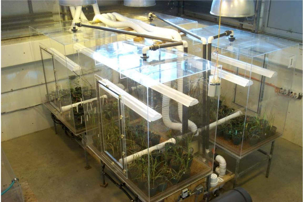
Figure 1. A 4-chamber, greenhouse-based CO<sub>2</sub> exposure system was constructed at the Alberta Research Council, Vegreville, Alberta to conduct studies on the effects of elevated CO<sub>2</sub> on crops and weeds.
