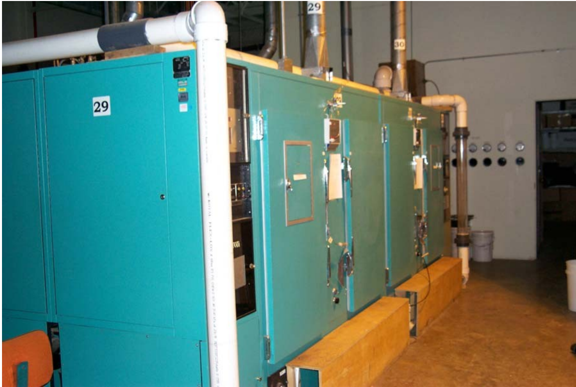
Figure 2. Six-chamber exposure system at ARC, Vegreville. Conviron growth chambers were previously modified for ethylene experiments and were retrofitted for use as a \text{CO}_2 system.
