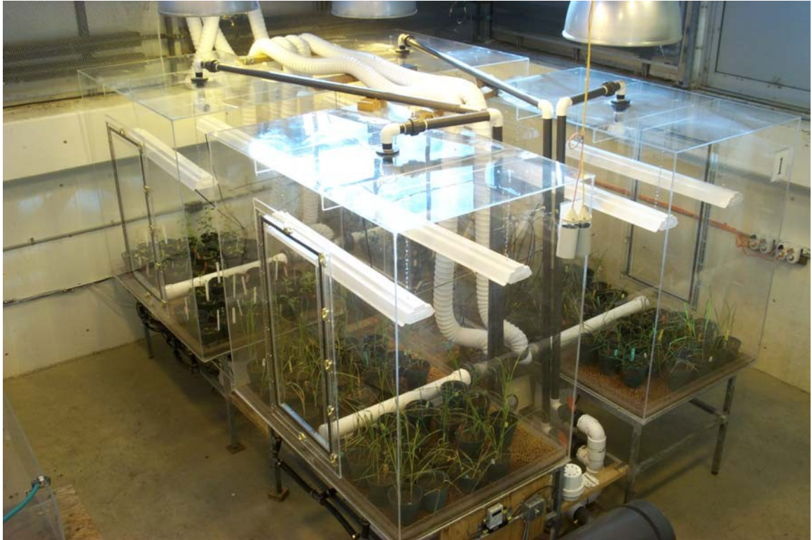
Figure 1. A 4-chamber, greenhouse-based CO 2 exposure system was constructed at the Alberta Research Council, Vegreville, Alberta to conduct studies on the effects of elevated CO 2 and weeds.
