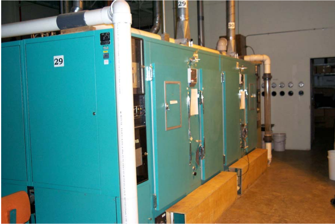
Figure 2. Six-chamber exposure system at ARC, Vegreville. Conviron growth chambers were previously modified for ethylene experiments and were retrofitted for use as a CO 2 exposure system.
